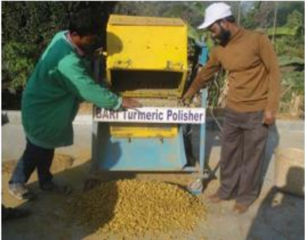
Figure 1.2: Discharging of turmeric from the polisher
